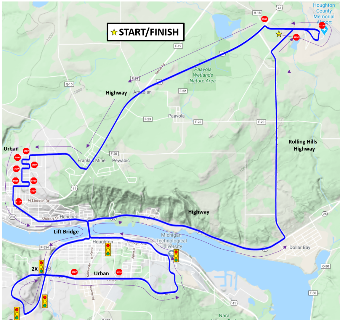
Figure 3.14: MTU Drive Cycle route overlaid on a map with directions, stop signs and traffic signals
