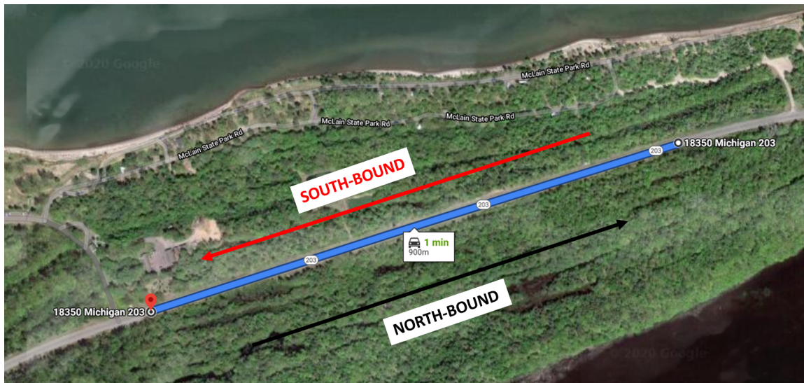
Figure 3.6: 900 m long route selected for Vehicle Platoon Testing on M-203 near McLain State Park
